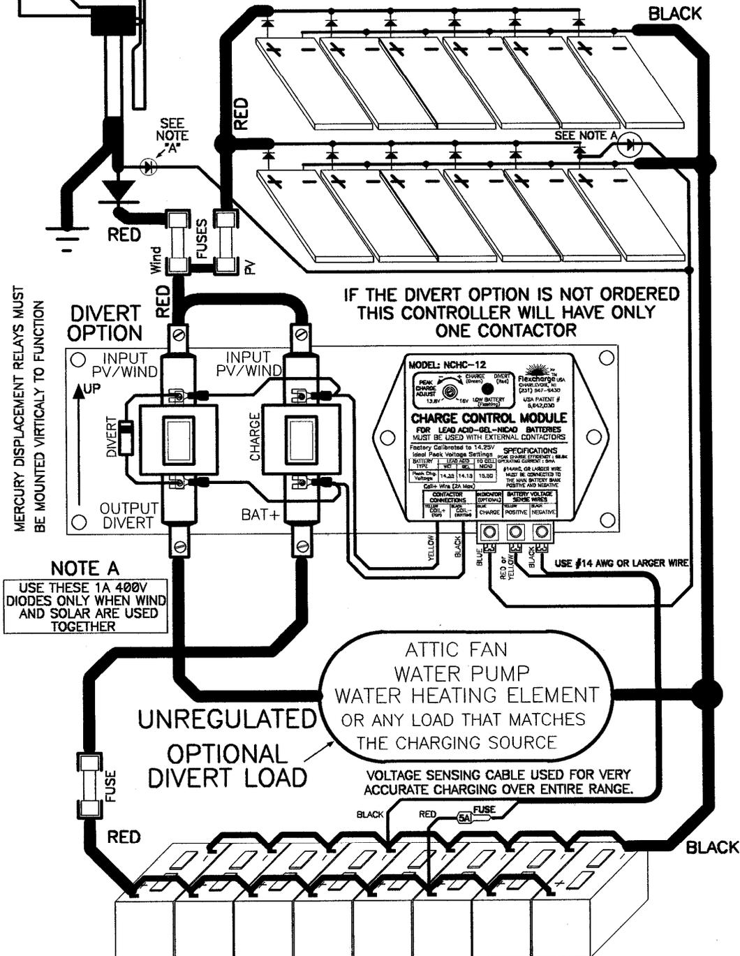
12V System is shown. Different voltage systems will require that the solar panels and batteries be wired appropriately.
